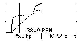
The power torque graph shows the relationship between horsepower/torque and engine RPM. The vertical axis shows the power and torque. The horizontal axis shows the engine RPM.
