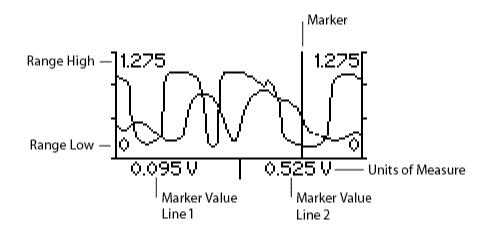
The data is sampled in 256 bursts of 1mS per sample. Recorded data stored to the SD card and opened using the Dyno-Scan for Windows software will show each 256-sample burst separated by a few hundred milliseconds.
