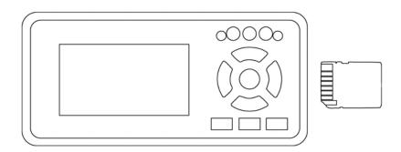
Plug the OBD II cable into the DashDyno OBD II port. Plug the OBD II connector into the vehicle's OBD II data port. The DashDyno will immediately power on when plugged into the vehicle.
