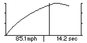
The acceleration graph shows the relationship between vehicle speed vs. time. The vertical axis shows the vehicle speed in MPH. The horizontal axis shows the time in seconds.
