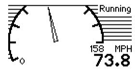
9 The acceleration screen will record up thought the <sup>1</sup>/<sub>4</sub> mile. It will terminate automatically if the vehicle begins to slow down or the maximum test time has expired.
