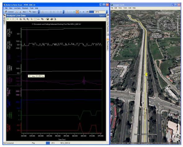
When a DashDyno live data file containing GPS data is opened, Google Earth draws a yellow line showing the complete vehicle path and zooms to that location. Moving the data cursor on the Analyze Live Data screen causes Google Earth to immediately fly to the new location on the yellow line. The Google Earth yellow pushpin shows the current GPS location within the data file.
