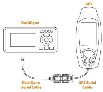
Your GPS receiver must be configured to output serial data. A setup menu on your GPS receiver will enable the NMEA output and a communication baud rate. Ensure the baud rate selected on your GPS receiver matches the DashDyno baud rate set at the Preferences > GPS Baud Rate menu.
