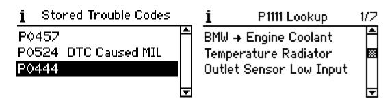
All diagnostic trouble code definitions are stored on the external memory card. The definitions must be located within the card directory \DTC for the software to locate the definitions.
